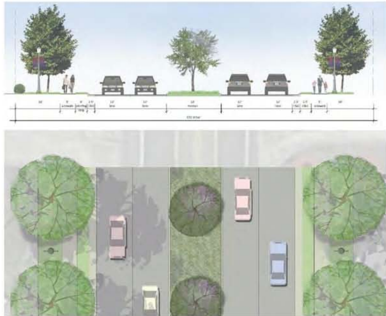
Figure 7. Cross-section of 4-Lane Divided Complete Street
