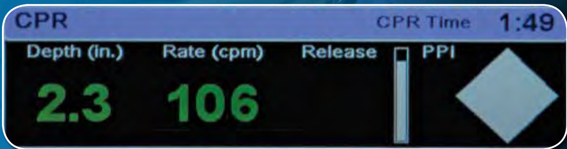
CPR Dashboard is a real-time window on the key metrics of high-quality compressions.
