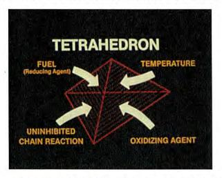
The first component of the tetrahedron is fuel. Fuel can be any combustible material such as: solid (such as wood, paper, or cloth), liquid (such as gasoline) or gas (such as acetylene or propane). Solids and liquids generally convert to gases or vapors before they will burn.
